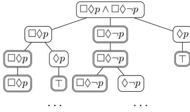
Figure 1: An accepting run of an ABA for  $\Box\Diamond p \wedge \Box\Diamond\neg p$  over an infinite sequence of states in which the truth value of  $p$  alternates. Double-line ovals are accepting states/conditions.
